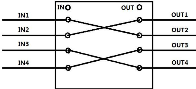
Remark: Inputs IN1 to IN4 can be freely switched to outputs OUT1 to OUT4. Two or more input channels cannot be selected simultaneously for the same output channel.
